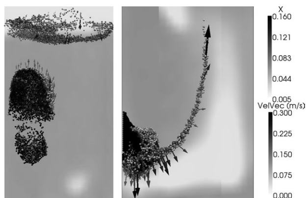
Figure 6. Biomass particles inside the dense bubbling sand bed during the drying process for u_0 = 0.365 m/s (left) and u_0 = 0.76 m/s (right).
